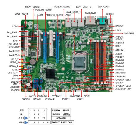
**Board Layout: Jumper and Connector Locations**
