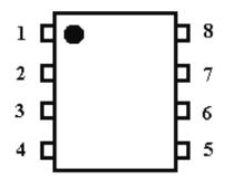
Figure 1. Package Type SOP-8
