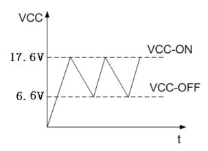
Figure 7. VCC-ON and VCC-OFF
