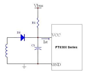
Figure 6. Start-up Circuit
