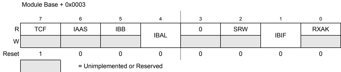
Figure 20-7. IIC Bus Status Register (IBSR)
