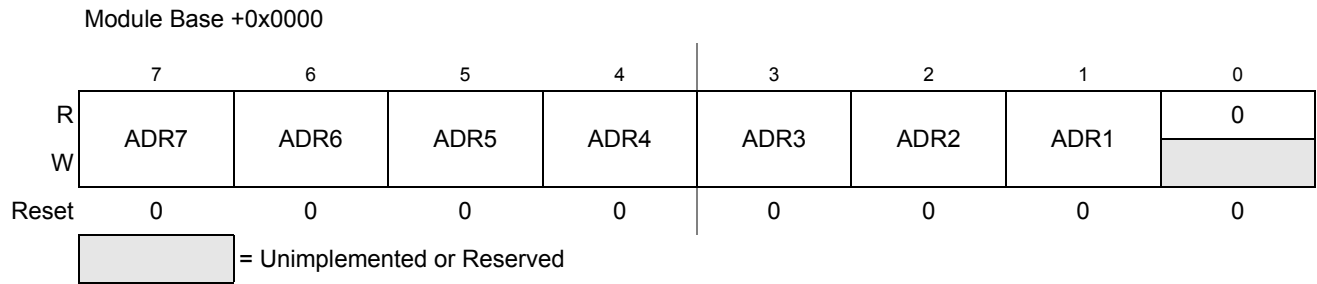
Figure 20-3. IIC Bus Address Register (IBAD)
