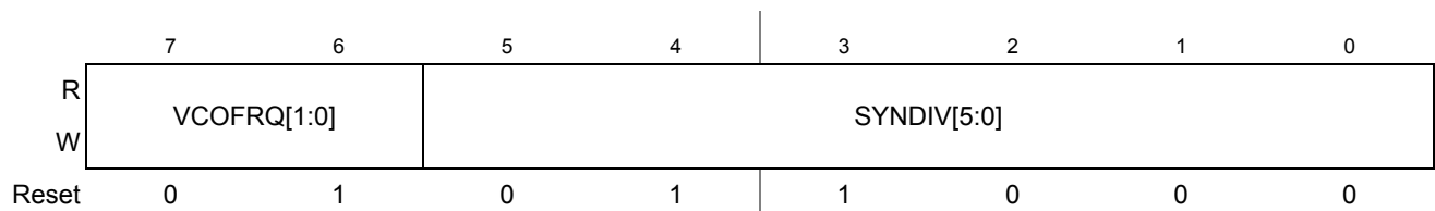
Figure 9-7. S12CPMU_UHV Synthesizer Register (CPMUSYNR)
