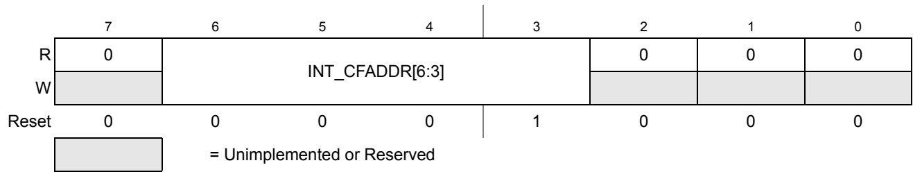
Figure 6-4. Interrupt Configuration Address Register (INT_CFADDR)
