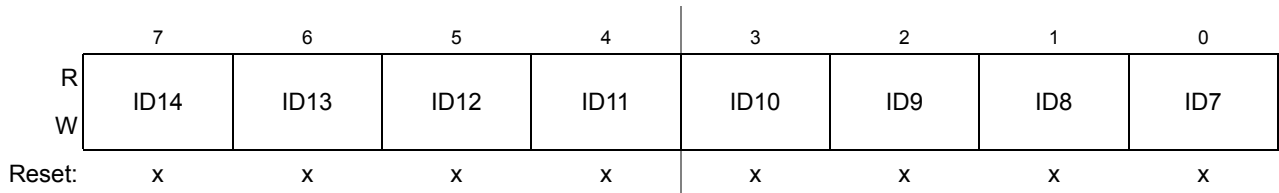
Figure 13-27. Identifier Register 2 (IDR2) — Extended Identifier Mapping
