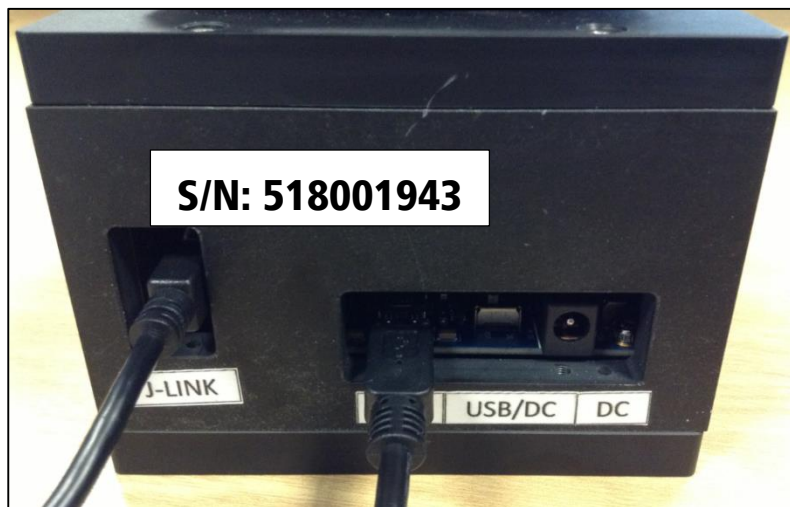
Figure 7: J-LINK cable connecting to programming jig
