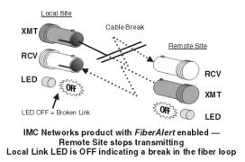
connection will go out indicating a fault somewhere in the fiber loop. Using FiberAlert, a local site administrator is notified of a fault and can quickly determine where a cable fault is located.
