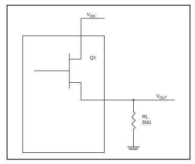
Figure 6. HSTL Driver Circuit and Termination
