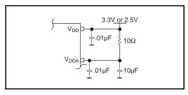
Figure 3. Power Supply Filtering
