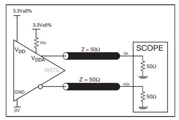
3.3V HSTL Output Load AC Test Circuit
