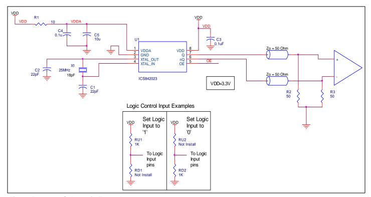
Figure 5. 842023 Schematic Example
