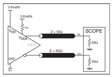
2.5V HSTL Output Load AC Test Circuit
