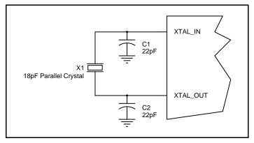
Figure 1. Crystal Input Interface
