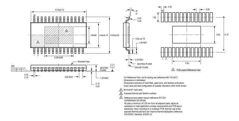
Figure 18: Package LP, 28-Pin TSSOP with Exposed Thermal Pad
