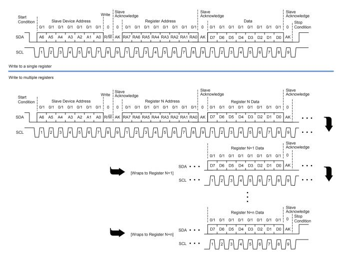
Figure 16: Writing to Single and to Multiple Registers
