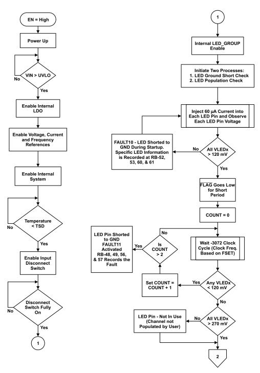
Figure 4a: Startup and Fault 11 Detect Flow Chart
