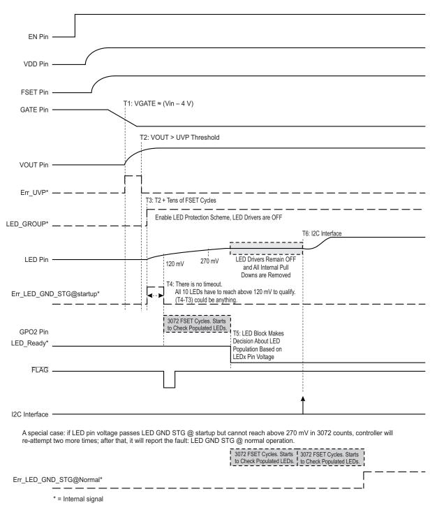
Figure 4c: Startup Timing Diagram
