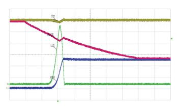
Case 2. Output-to-GND short fault occurred before startup
