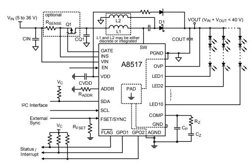
Application C: The A8517 can be used in a SEPIC (Single-Ended Primary Inductor Converter) Configuration
