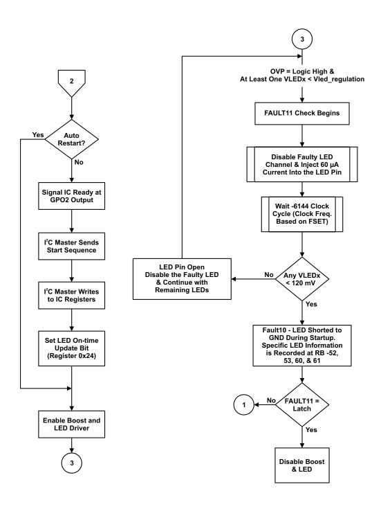
Figure 4b: Startup and FAULT11 Detect Flow Chart (Cont.)
