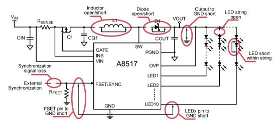
Figure 8: Examples of System Fault Modes
