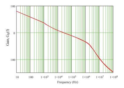
Figure A-4: Plot of the Whole System Closed Loop Transfer Function Gain versus Frequency, with a Cross Over Frequency, f<sub>C</sub>, of 30 kHz
