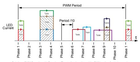
Polyphase PWM Operation with Grouping – The starting time slot and the PWM on-time for each group is determined by the time slot and the on-time of the lowest-numbered channel within that group, so all LED channels in the same group turn-on and turn-off together. Each time slot is sequential and periodic, and unused time slots are maintained. Any individual phase can overlap later time slots. The LED current for each channel is individually programmed, regardless of grouping.
