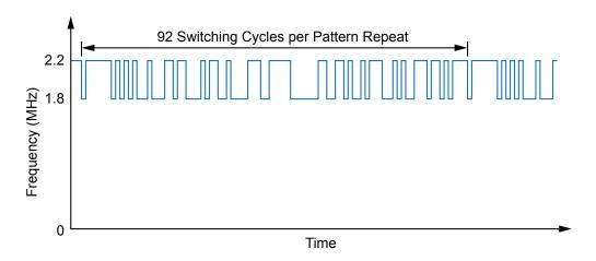
Figure 5: A8517 Dithering Scheme at 2 MHz ±10% (frequency jumps between 1.8 MHz and 2.2 MHz, as governed by a 46-bit pseudorandom pattern)
