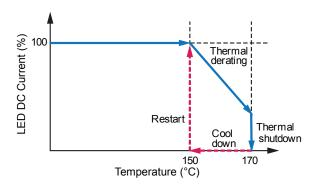
Figure 9: Thermal Derating and Shutdown Protection Features
