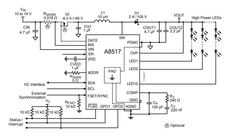
Figure 11: Schematic Diagram Showing Calculated Components from the Above Design Example
