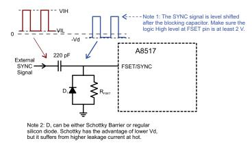
Figure 2: Low FSET\_SYNC Signal Fault Counteraction Circuit
