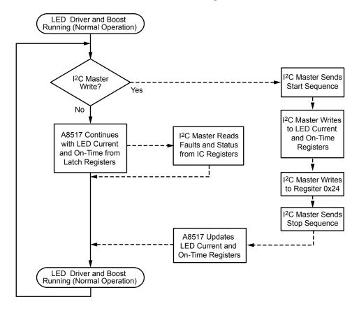
Figure 13. I<sup>2</sup>C Interface During Normal Operation
