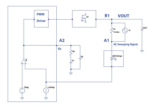
Figure A-5: Simplified Block Diagram for the Closed-loop Whole System to show how to measure the gain of the power stage or closed-loop system gain and phase margin
