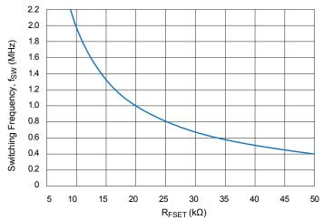
Figure 1: Switching Frequency versus Value of the R<sub>FSFT</sub> Resistor
