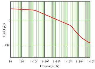
Figure A-1: Plot of Power Stage Transfer Function versus Frequency
