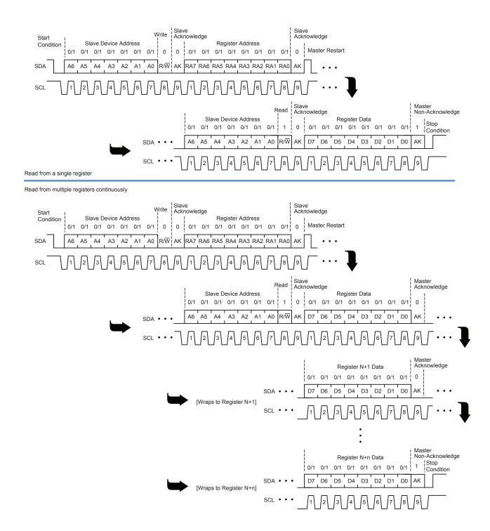
Figure 17: Reading from Single and to Multiple Registers
