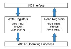
Figure 12: I<sup>2</sup>C Interface Communication Structure
