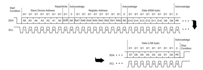
Figure 15: Complete Data Transfer Pulse Train
