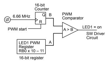
Figure 3: PWM On-time Comparator Circuit
