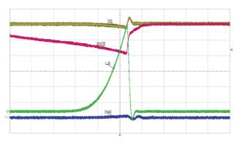
Case 3. Output-to-GND short occurred during normal operation
