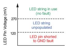
Figure 10: A8517 LED Short-to-GND Check Before Startup
